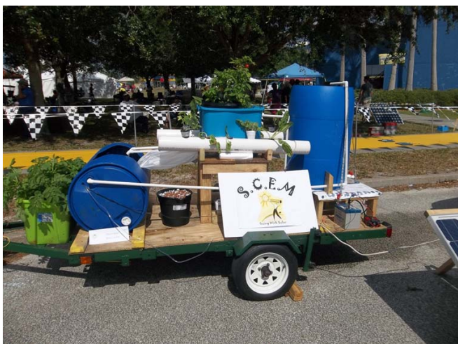
The SCEM - Self Contained Eating Machine, a sustainable aquaponic system
