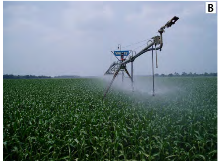
Figure 11. Land application of solids using a manure spreader (A) and liquid effluents through a center pivot irrigation system (B).
