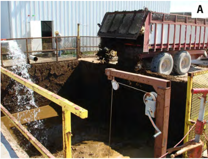
Figure 8. (A) Manure and bedding mixture is being loaded into (B) the mixed plug-flow anaerobic digester (biogas is unloaded at the far end).
