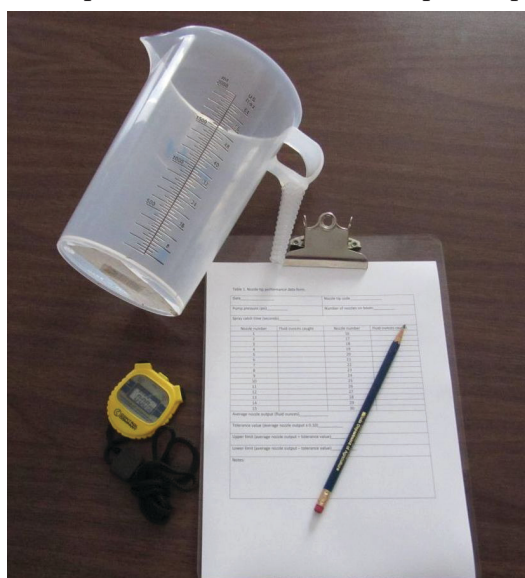
Figure 2. Simple items needed for performing a nozzle performance test.
