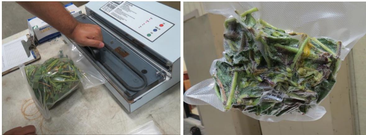
Figure 2. (Left) Vacuum sealer used to ensile the vines; (Right) One replicate sample of ensiled sweetpotato vines used in the silage trial
