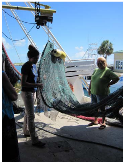
Cinthia Sandoval with Wild Ocean Seafood Market shows participants a commercial shrimp net, including the required turtle excluder device.
