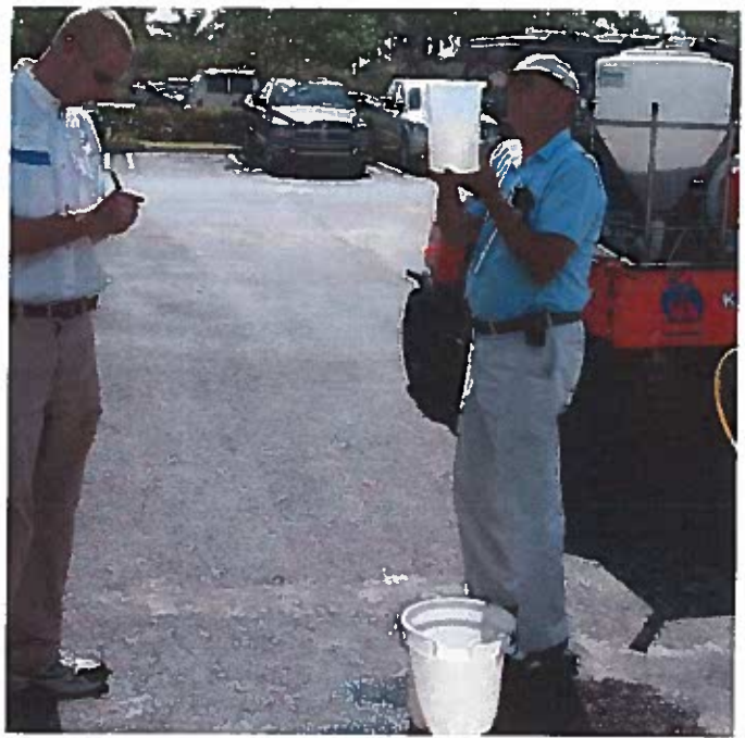
Figure 5. The number of ounces collected from the calibration nozzle is equivalent to the GPA. Credits: UF/IFAS Pesticide Information Office
