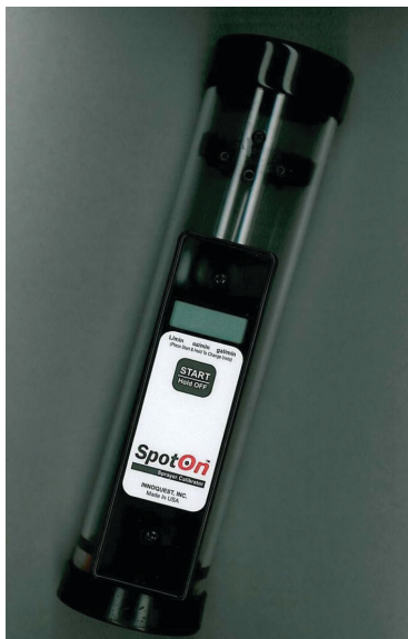
Figure 1. Commercially-available flow meter for testing tip output. Credits: UF/IFAS Pesticide Information Office
