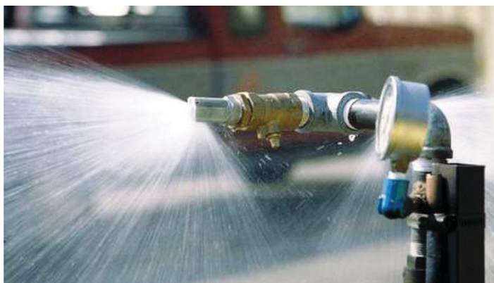
Figure 2. A wide-swath, boomless nozzle. Credits: J. Boyd, U. of Arkansas
