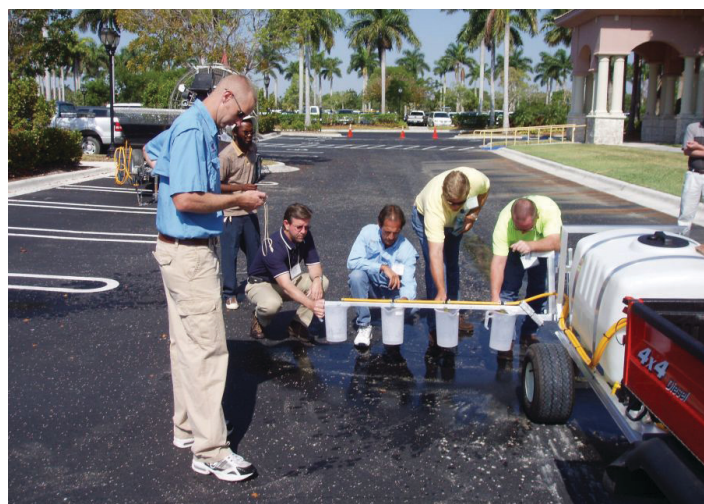
Figure 3. Performing a nozzle output check. Credits: UF/IFAS Pesticide Information Office
