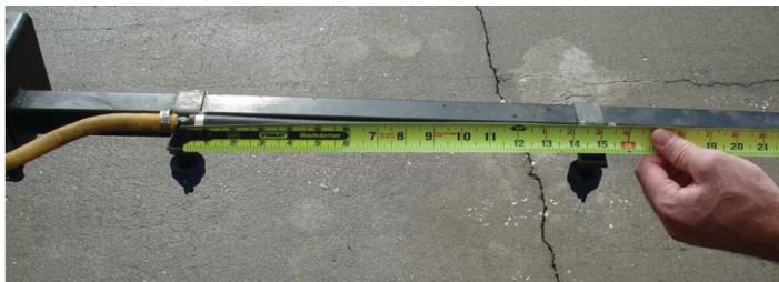
Figure 1. Measuring nozzle spacing to determine “W”. Credits: J. Ferrell, UF/IFAS
